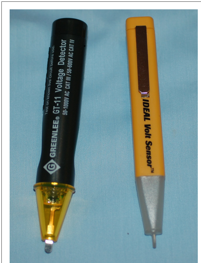
Accident Greenlee NCVD on the left, Exemplar IDEAL NCVD on the right.
